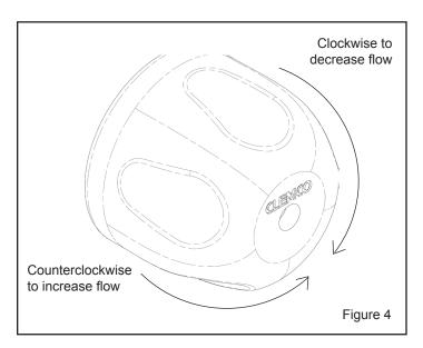
3.4 Optimum abrasive flow depends on the type and size of abrasive and blasting pressure, and is best determined by experience. Use as little abrasive as possible while maintaining the maximum cleaning rate. The air/abrasive mixture should be mainly air. As a rule, the stream of abrasive coming out of the nozzle should barely discolor the air when seen against a contrasting background.
